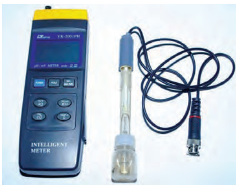
Fig.1.3: Digital pH meter
